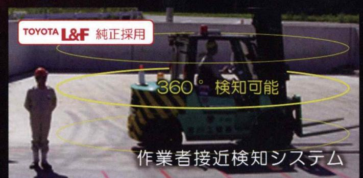
RFID [Radio Frequency Identification]
