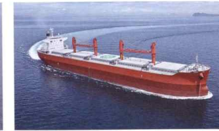
63,000M.T. D/W TYPE BULK CARRIER (L)199.98×(B)32.24×(D)19.15
