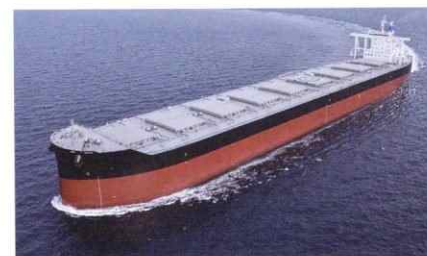
183,000M.T. D/W TYPE BULK CARRIER (L)291.95×(B)45.0×(D)24.7
