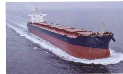
81,000M.T. D/W TYPE BULK CARRIER (L)228.94×(B)32.24×(D)20.0
