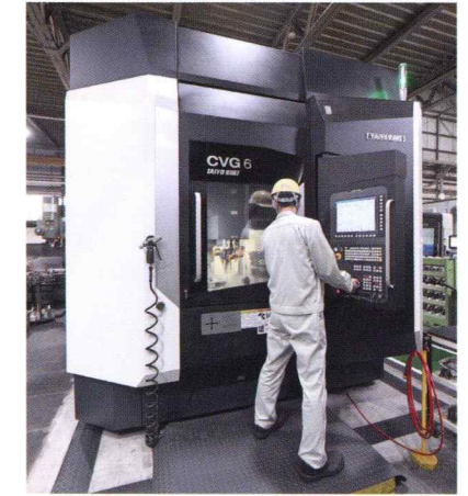
CNC 立形複合研削盤 / CNC vertical multi axis Grinder
