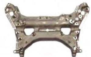
量産製品形状 Modified part shape suitable for mass production
