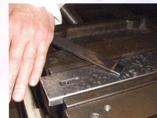
キサゲ加工による油溜り作成 (工作機械向けギブ) Oil Reservoir Created by Scraping (Machine Tool Gib)
