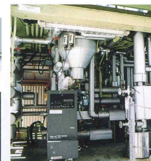
生分解性ポリマー重合設備 Polymerization pilot plant for biodegradable-polymer
