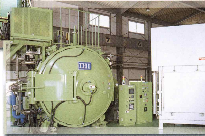
世界トップクラスの能力を持つ真空焼入炉(左)と焼戻炉(右) Vacuum hardening furnace (left) and tempering furnace (right) with world's top level performance
