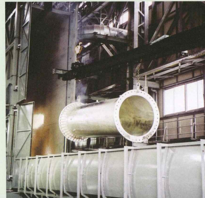
▲めっき上り Just lifted up from the zinc bath
