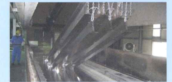
▲めっき加工 Hot dip galvanizing
