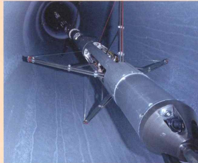
▲管内めっき厚測定用/塗装用ロボット Robot for measuring inner zinc coating thickness and for painting
