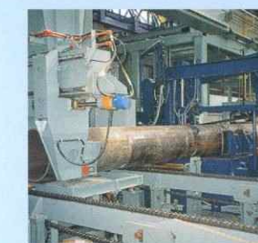
▲NC主材切断装置 NC cutting machine for tower main post members
