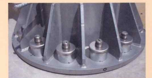
▲ボルト抜け防止金具 (デンロック) Bolt-dropping protection hardware called "Denlock"
